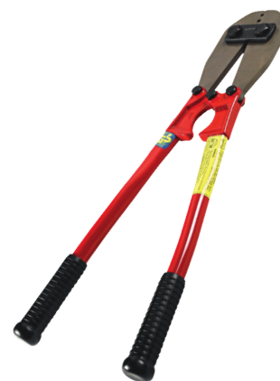
Mechanical WDS tong for crimping 3 and 4 mm small fittings on flexible wire 7x7 and 7x19 construction.
