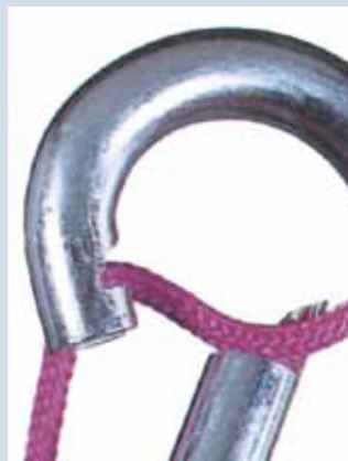
OLD 2 hooking points 2 sharp edges
