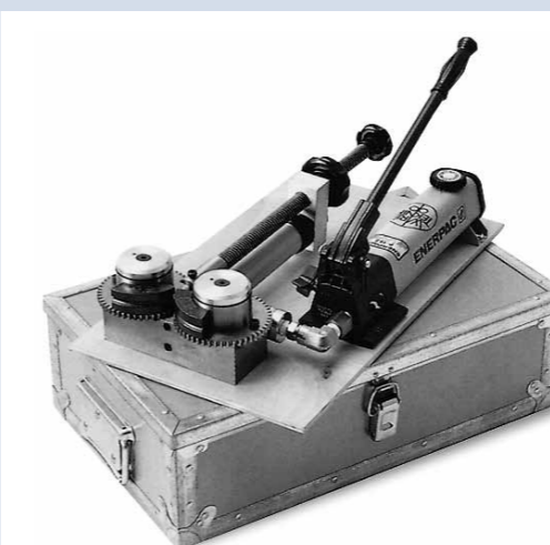
Wiretechnik swagingmachine A 100 incl. roller dies 2,5-3-4-5 mm, handpump, tools and transportbox
